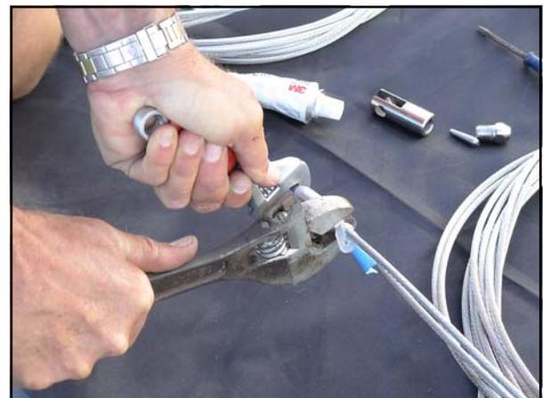
use a wrench to tighten but don't use anything longer than six inches to crank the fitting down. Too much force could deform the relatively soft 316 stainless steel fitting and render it unsuitable for re-use later. Sealant should squeeze out around the wire at the base of the fitting. Wipe the excess off with a rag. Good job. One down, nineteen more to go.
