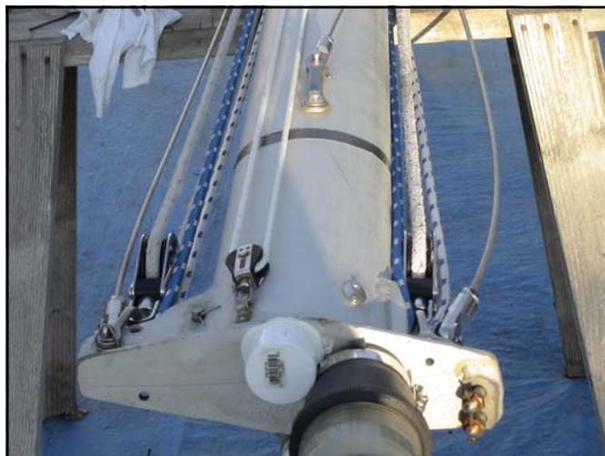
*With the mast down, the author took the opportunity to rig blocks for topping lift and spare jib halyard, taking advantage of the hollow pins used for the stay toggles.*
